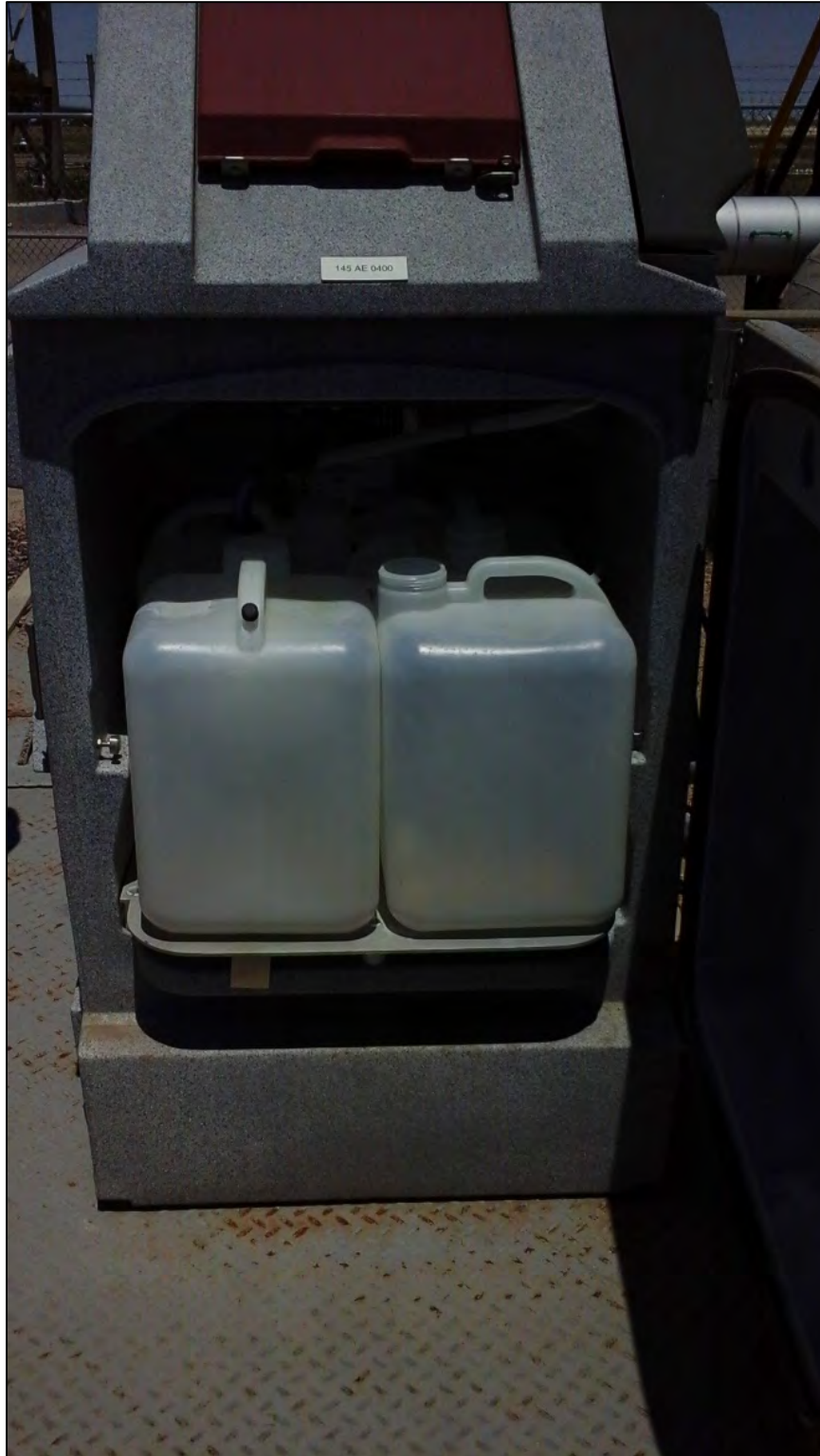
Photograph 6. View inside the ISCO automatic composite sampler at Outfall 003B. This sampler was not equipped with an independently calibrated thermometer.
